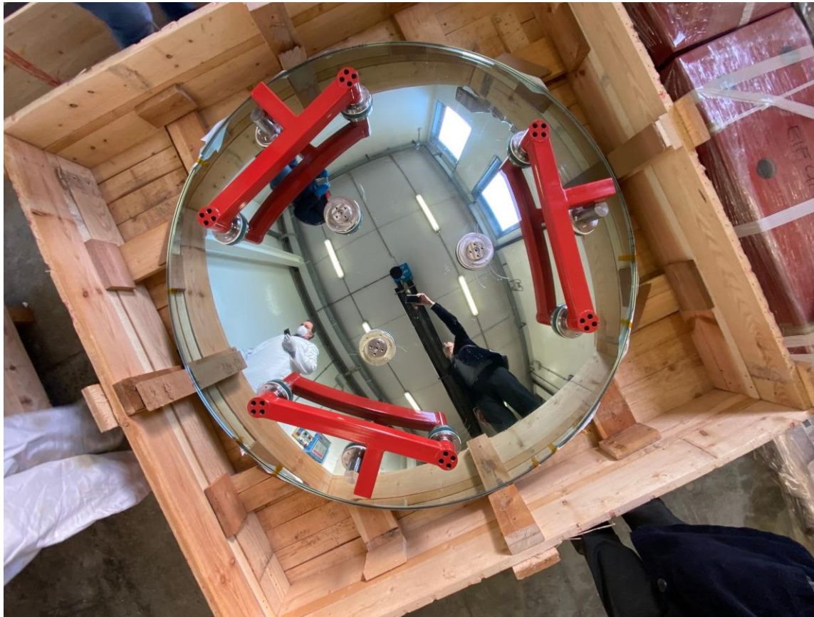
Gluing M2 tangential pads @ telescope integration site
