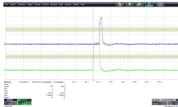
**Double pulse resolution** ~10 ns per channel and < 10 ns between different channels
